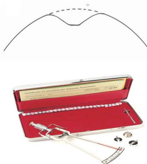
Fig 1: Corneal deformation in indentation tonometry (a); the instrument (b)
